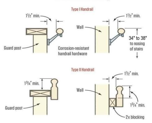
**Note:** A 2x4 or 2x6 is not acceptable without recessed areas on both sides as shown above.
