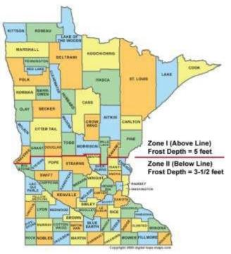
Paragraph 5.1 of ESR-1895 states that the system must be installed in accordance with the published installation instructions. The installation manual defines the frost depth equivalence shown above as 48" deep for the DP50-50" model and 60" deep for the DP75-63" model. This is shown in the Diamond Pier installation manual on page 6; and is supported by the statement in paragraph 2.0. for use in all weathering classifications.
