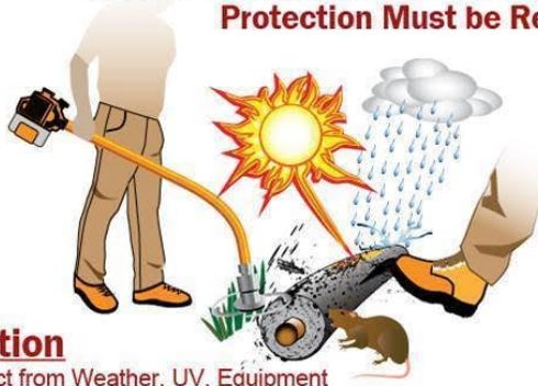
Damaged Insulation from landscape maintenance
